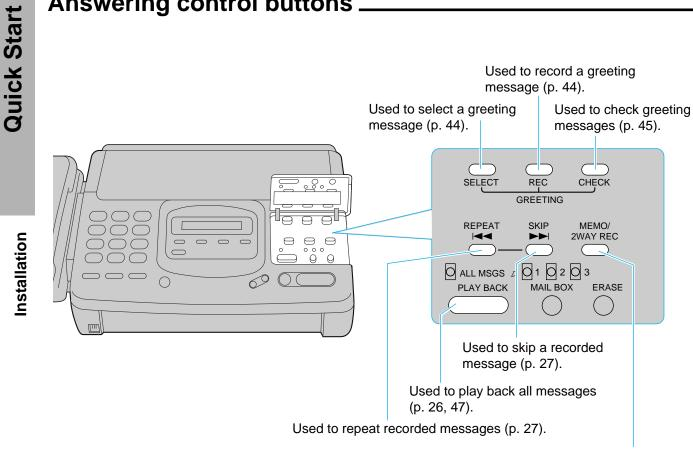
Used to record a memo message (p. 28). Also used to record a telephone conversation (p. 28).
